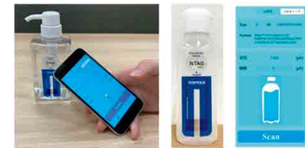
NFC tag that detects liquid volume
