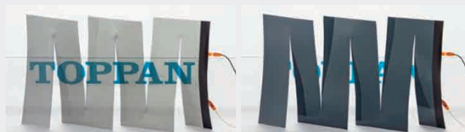
LC MAGIC™ Normal Black can be cut into any shape and has visible light transmission of 43% when power is on (left) and 5% when power is off (right).
